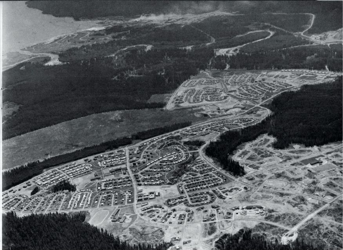
Airview shows "U" shaped crescents in Kitimat's planned neighborhoods. Crescents provide privacy and limit automobile traffic.
