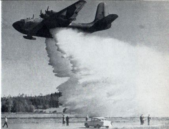
7,000 gallons of water in one drop! Modern fire prevention in the woods has had a big assist from the Flying Tanker operated by a group of B.C. forest industry companies, of which MacMillan, Bloedel and Powell River is a major participant.
