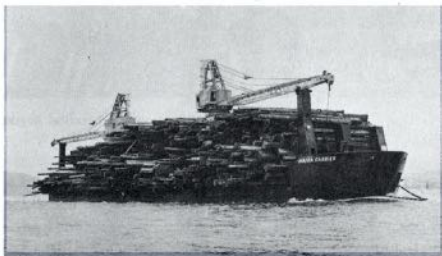
Transportation of logs by barge has speeded deliveries reducing time logs are in water with resultant reduction in waste by tereid infestation.
