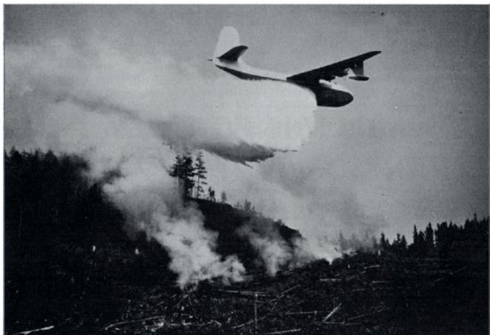
Mars Water Bomber in actual operation unloads its full 6,000 gallons to quickly curb forest fire.
