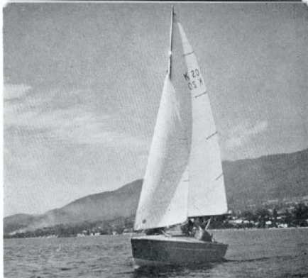
Centreboard Sloop built with fir plywood panels sails smartly across English Bay.
