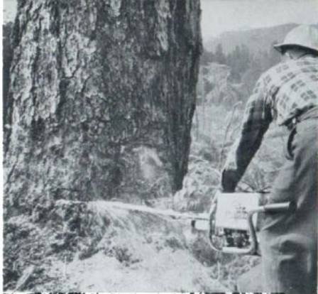
Falling by power saw has speeded production and reduced waste to a minimum.
