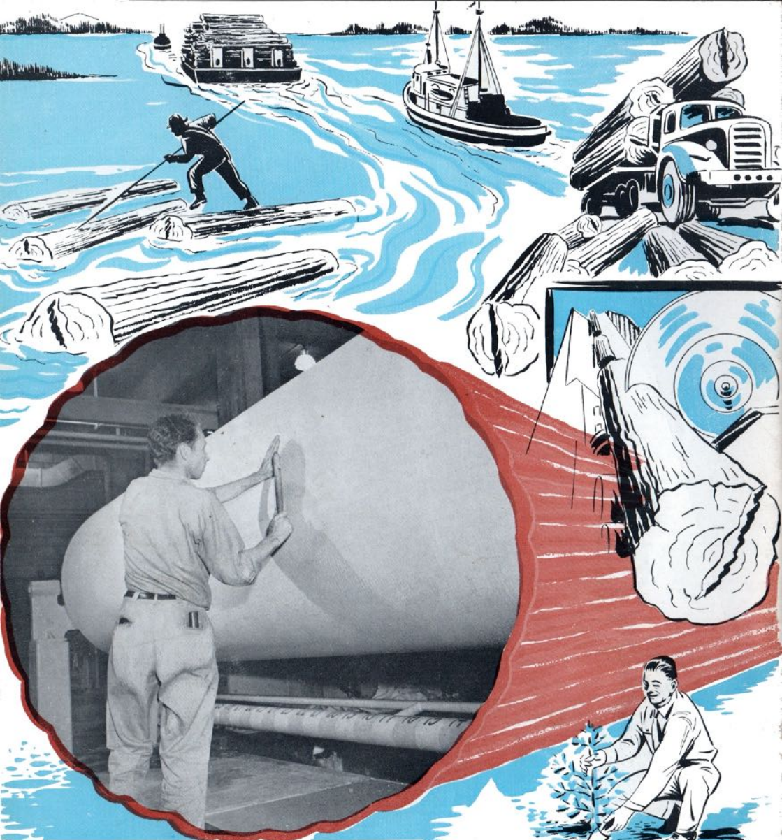
Newsprint coming off the huge machines onto the reels is carefully checked by the backtender to ensure uniformity and maximum printing quality.
