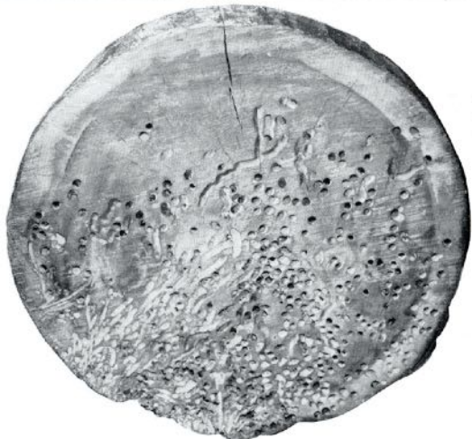
Typical section of a teredo infested log.
