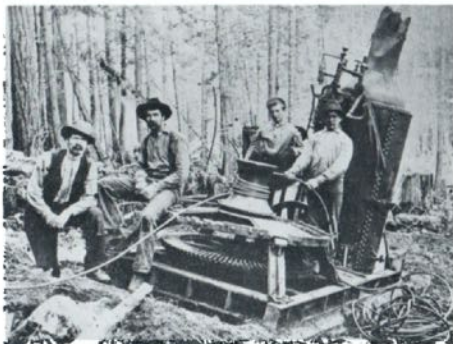
First steam donkey in British Columbia was operated at Chemainus in 1902.
