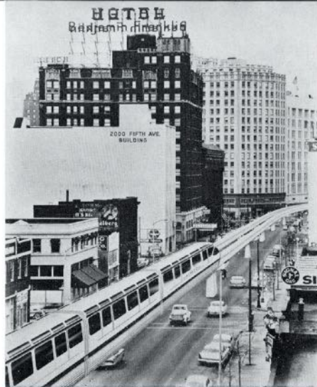
Century 21 - Alweg Monorail, world's first high speed mass transit monorail, is now being built to serve Century 21 Exposition. Shown here is an artist's conception of one of the two four-car trains, on the 1.2-mile track between downtown Seattle and the Century 21 site.
