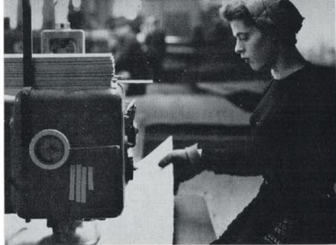
4 The fascinating patching machines where knots and other blemishes are punched out and replaced by solid wood.
