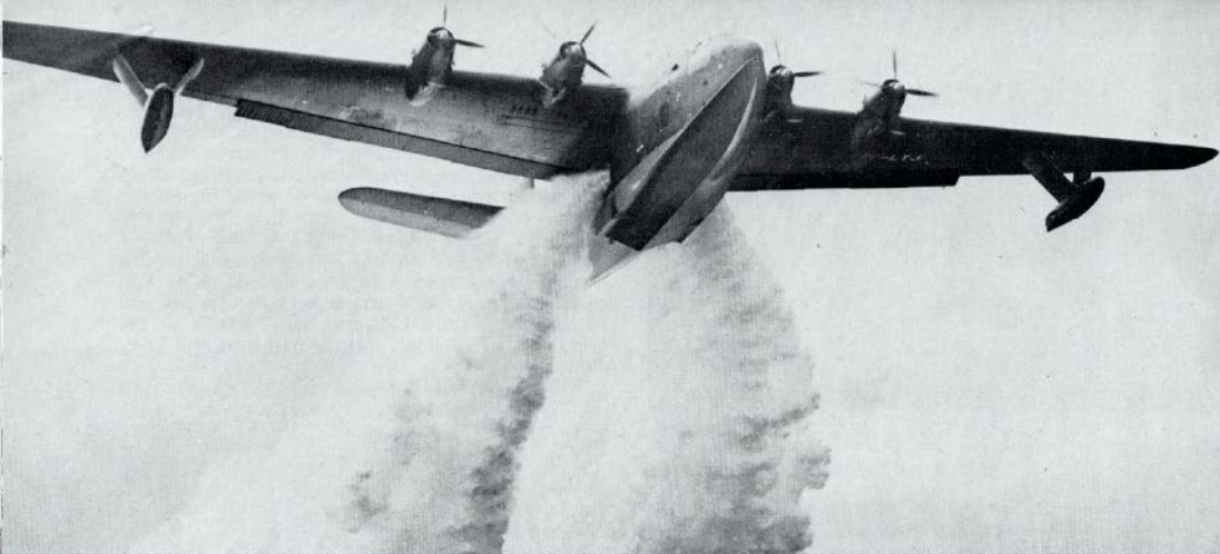
Water bombing by large aircraft, carrying up to 7,000 gallons of water, has been invaluable in fighting fires in inaccessible areas.
