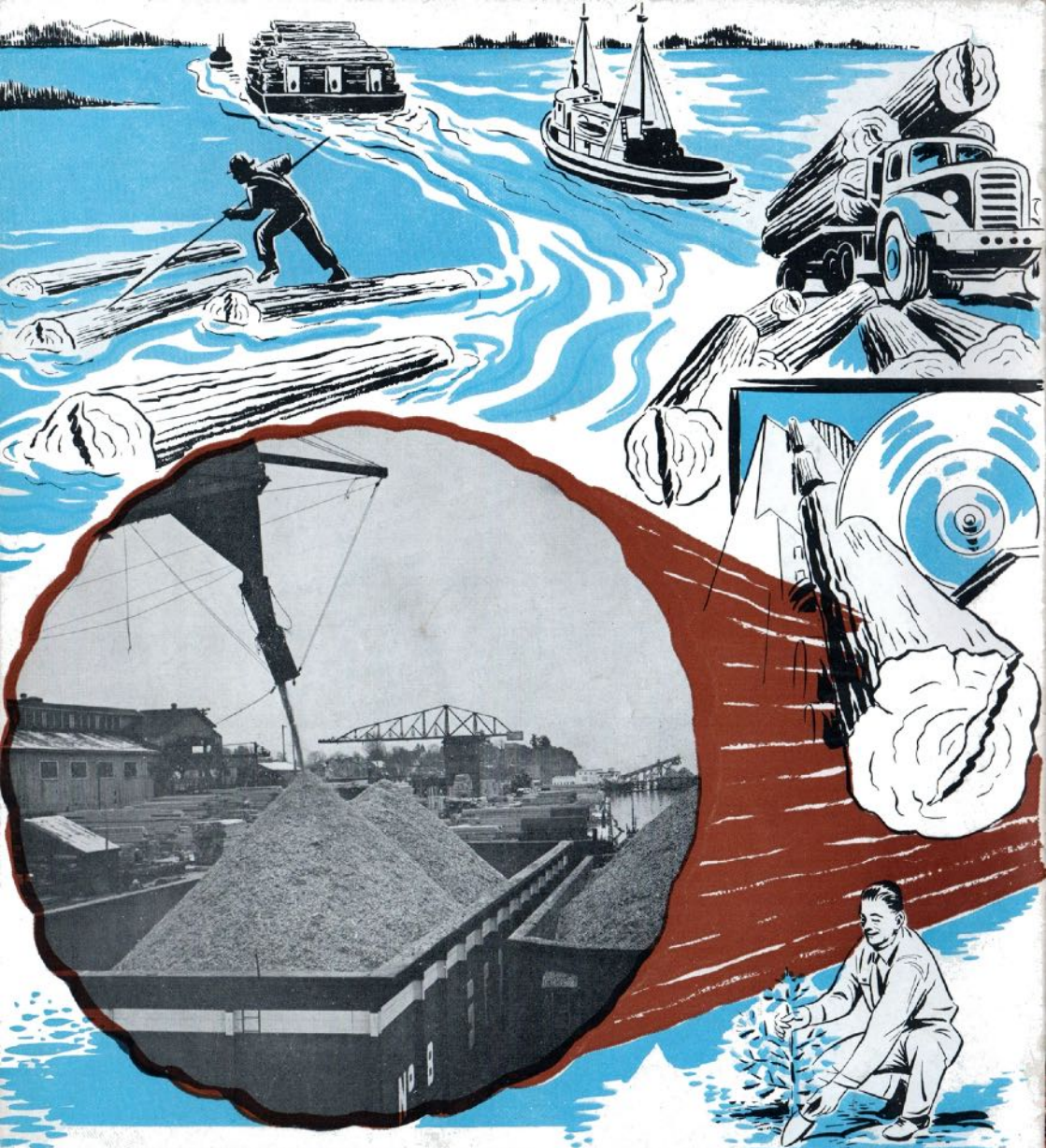
Chips from the Company's Canadian White Pine Division on the Fraser River being unloaded on barges for transportation to the Harmac Pulp Division near Nanaimo. Chipping facilities in the sawmills have enabled greater utilization of logs and reduced waste to a minimum.
