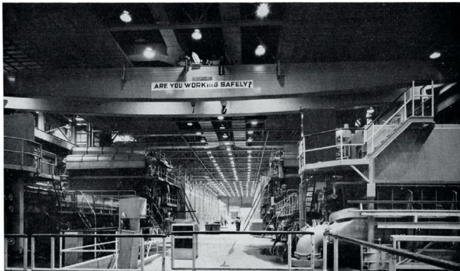
Two modern newsprint machines at Company's Port Alberni plant have a total capacity of 700 tons daily.
