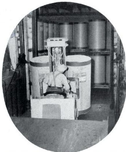
Wharf elevator at Powell River lowers jeep load of newsprint to covered barge at dockside.
