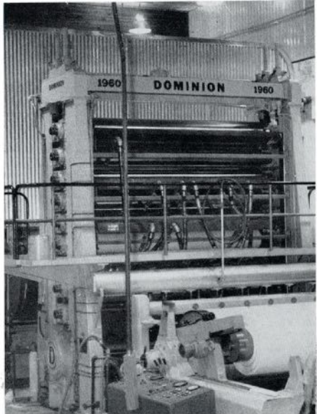
Calender stack and reel—dry end.
