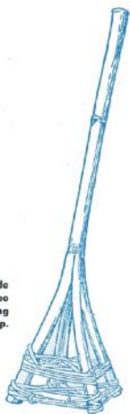
Churner made of bamboo for mixing the pulp.
