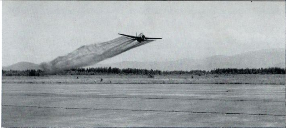
An "Avenger" plane releasing coloured dye for droplet pattern tests at Abbotsford airfield.
