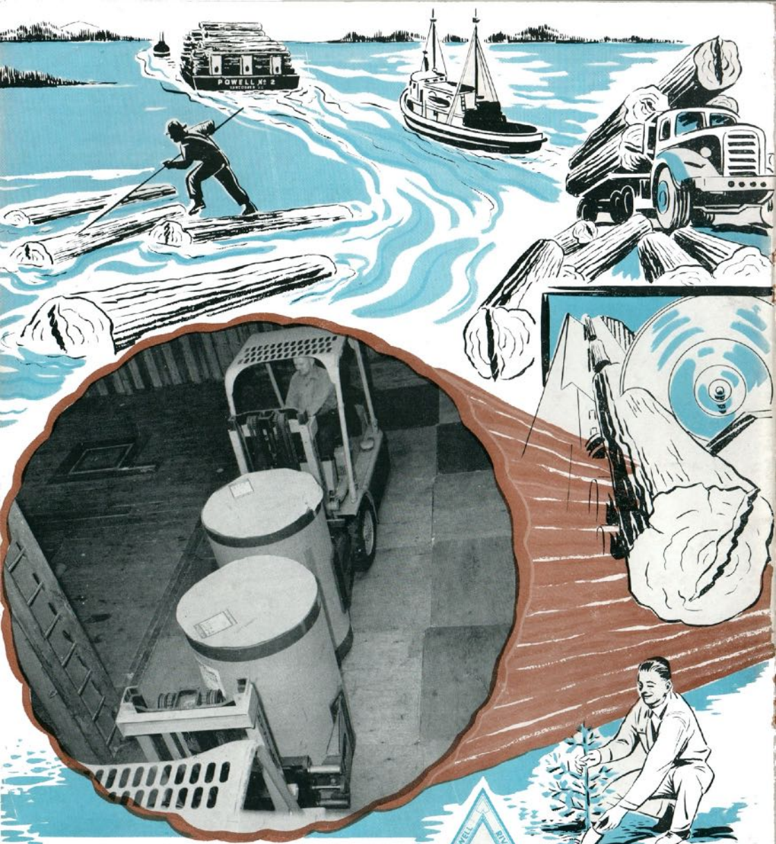
Labour-saving method of loading newsprint is shown above where jeeps operate in the hold of the ship, placing and stacking newsprint rolls.
