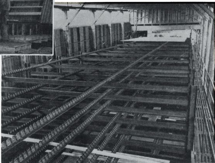
First views of the semi-automatic sorter-stacker at W.S.M. Random length lumber begins its climb to the sorter in picture at left. The various lengths are automatically conveyed at the different levels of the sorter (below) and stacked accordingly at the end of the line (third photo).
