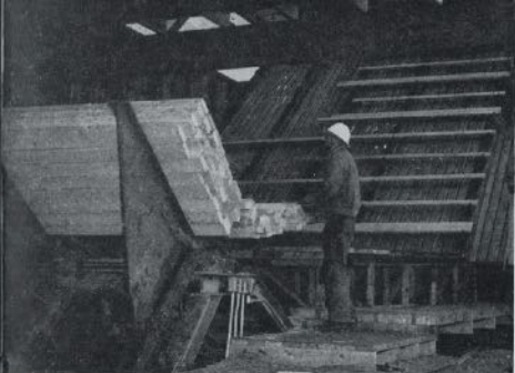
First views of the semi-automatic sorter-stacker at W.S.M. Random length lumber begins its climb to the sorter in picture at left. The various lengths are automatically conveyed at the different levels of the sorter (below) and stacked accordingly at the end of the line (third photo).
