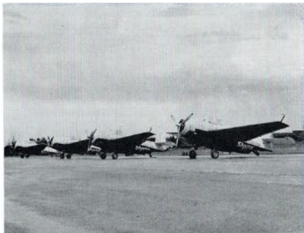
The four "Avenger" planes used for the spraying program, each carrying approximately 800 gallons of solution.
