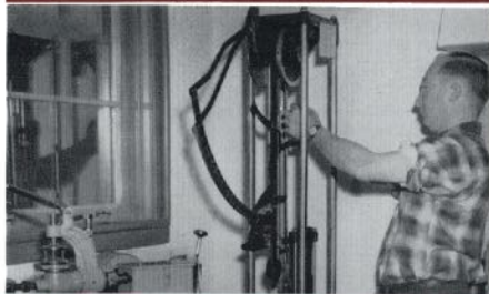
Bill Hayes operates tensile tester. Machine at left tests bursting strength of pulp.
