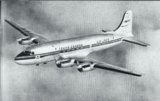
A Northstar 40-passenger airliner used by T.C.A. on trans-continental and overseas routes. Built by Canadair, Montreal.
