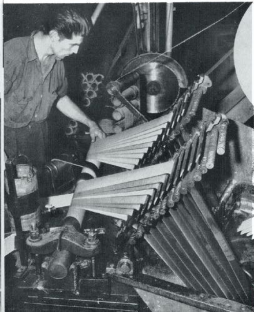
The Core Machine, with core strands passing through liquid glue.
