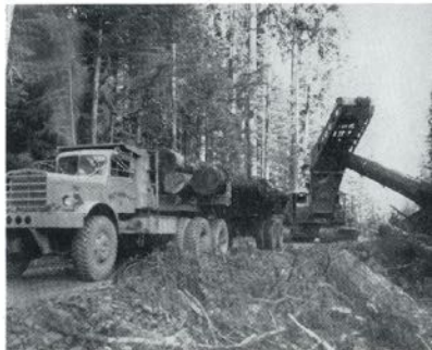
2 1/2 yard Lima shovel with steel goose neck boom loading logs on Kenworth 40 ton truck and 35 ton Columbia trailer.
