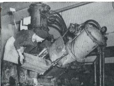
The pocket grinder now used in operations at Powell River.
