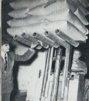
Harold A. Herzog (left) and Forrest Green, of Seattle, adopted this novel method of using cores as pallet boards. This load of flour weighs 2700 lbs.
