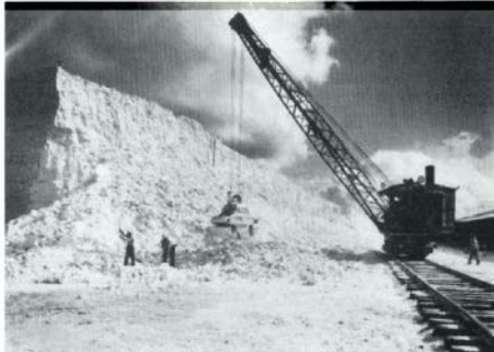
Loading sulphur from vat face at New Gulf, Texas.
