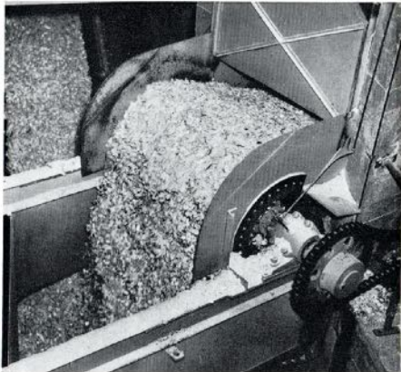
Thirty seconds later, this is how the same log looks. It is now a mass of uniformly sized chips.
