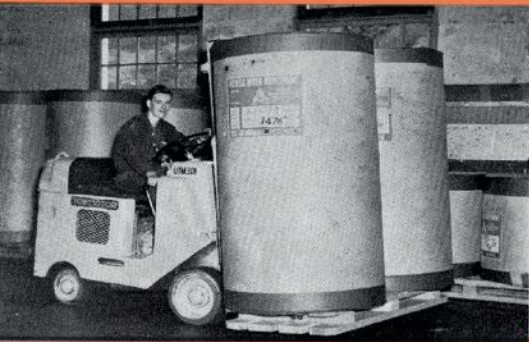
The jeep carries rolls from the weighing machines to waiting flatcars. This was formerly a hand-trucking job.
