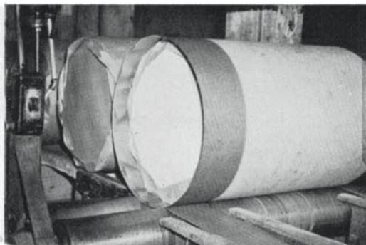
No. 2—The ends of the body wrap are crimped about the ends for initial protection (left).
