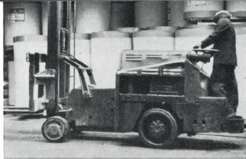
Jeep reaches floor, swings off elevator and deposits load.
