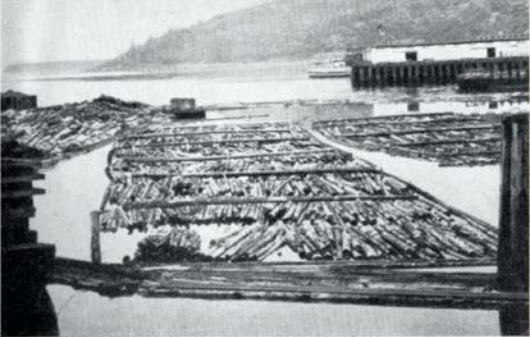
Bundles of small logs in a flat boom in the Powell River log pond prior to breakdown.
