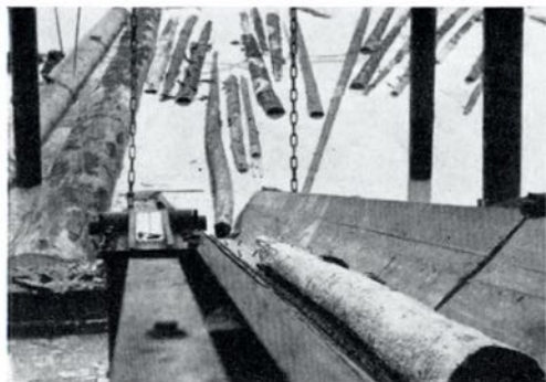
A small log coming up the jackladder with other logs in the selection pond below.
