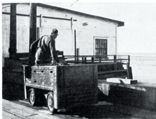
A miniature jeep, one of the fast-moving wharf jitneys for light equipment and transportation.
