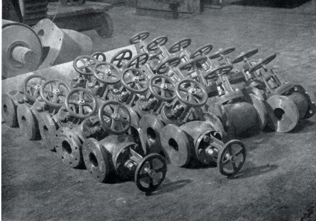
First shipment of 3-inch steam valves turned out in the Powell River machine shop.
