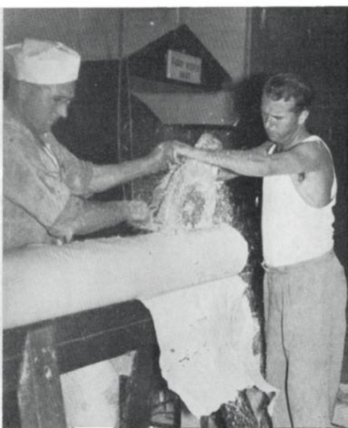
Millwright Foreman Theo Caron stands beside the wooden rodded Decker Screen, which replaces the former copper rodded equipment. The use of wood rods, introduced by Theo, has maintained the efficiency of operations and curtailed the use of vital copper.
