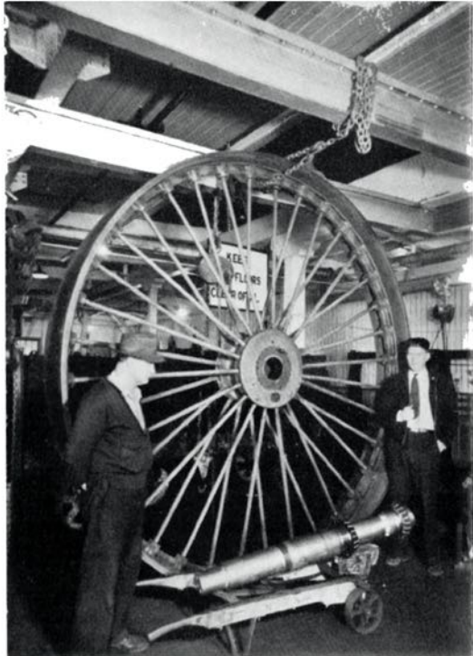
Ross Black, mechanical superintendent (right), and Tony Chiarcossi, stand beside the big 10-foot band mill wheel, renovated to fit local requirements. Below is the shaft, re-designed by our machine shop crew.
