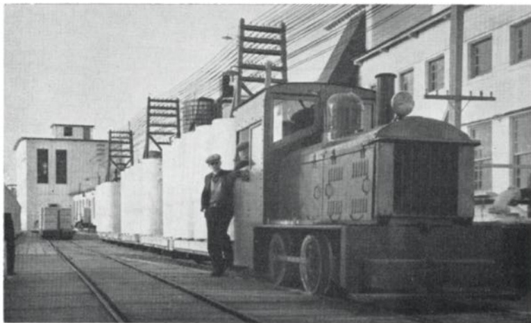
A Diesel Locomotive, with a "drag" of large newsprint rolls, passes along the grinder room front from storage shed to wharfside.
