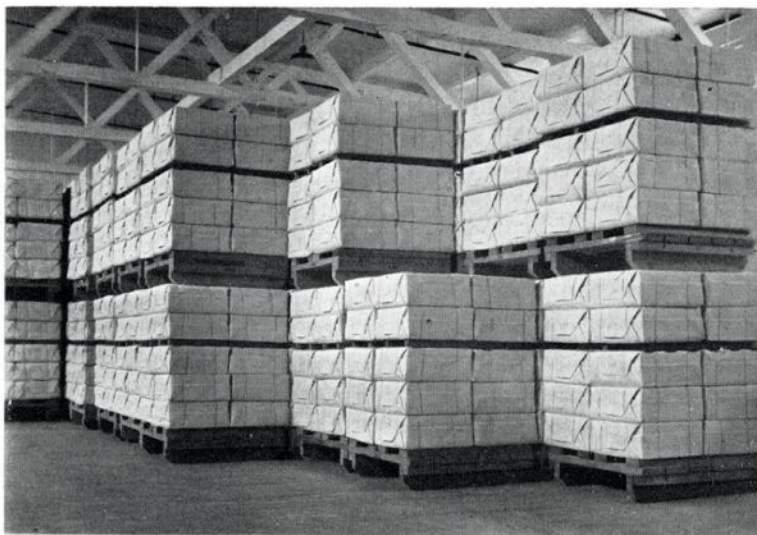
Bales of sulphite pulp in storage at Powell River, showing sturdy, neat compactness of the protecting wrapper.
