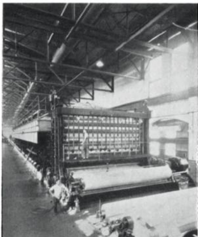
The Calender Stack on No. 7 machine, through which newsprint is being wound on to the reel at close to 1300 feet each minute.
