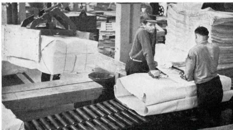
Wrapping up sulphite pulp. The pulp is carried along the rollers seen in the picture, wrapped and picked up by the boist seen in the upper left and transferred to waiting flat cars.
