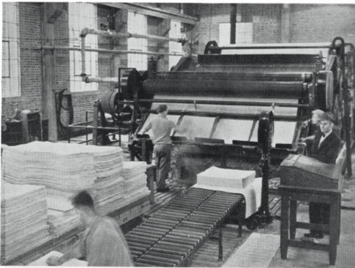
The Powell River Kamyr machine in action. The machine has a capacity for 100 tons of high-grade air-dried sulphite pulp daily. The Kamyr converts pulp to sheet form, cut to sizes ready for shipment. In the above, Al Watson, Sulphite Superintendent (right foreground) inspects the "run."
