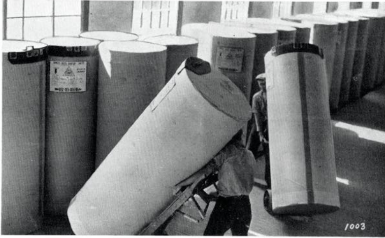
Rolls of newsprint being loaded on the waiting flat cars in the finishing room. The iron shields used to protect the roll against possible damage are clearly visible. The shield on the roll about to be placed on the cars will rub the shield on the car roll. Thus no actual contact of the paper takes place. The shields take up the shock of loading.
