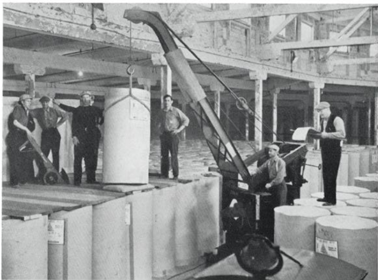
Careful handling of newsprint rolls in the storage sheds is shown in the above photograph. Craneman Alf Statbam lifts up the roll, under which a cushion is deposited to protect the edges from damage as it is lowered to the top deck.
