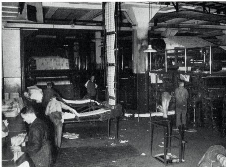
A section of the presses, showing the paper conveyors to the publishing department.
