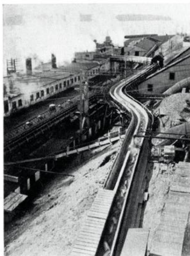
Blocks of wood, cut in pulping size, carried by flume to the grinder mill where the first stage of their conversion to pulp begins.
