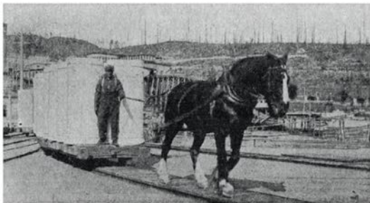
How they used to take paper from the mill to the wharf in the early days. This photo, taken in 1915, shows the old horse-pulled trains on the way to the sheds.
