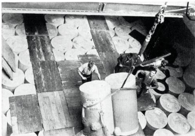
Stowing paper in the hold of the S.S. "Nordnes" at Powell River.
