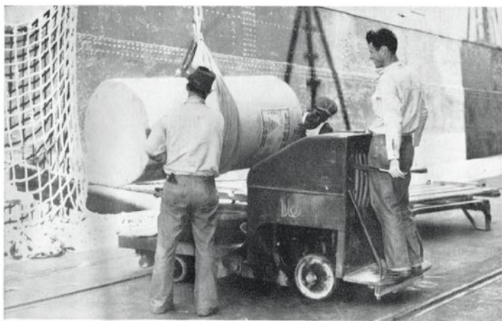
Powell River newsprint loaded direct from the ship's side to waiting motor trucks. This method of handling will prove of interest to Powell River wharf employees.
