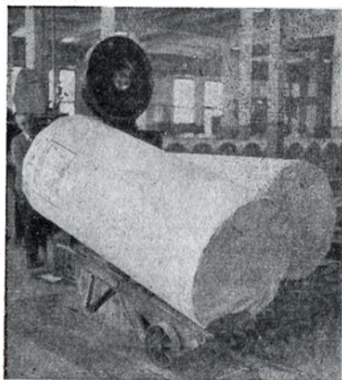
Rolls of newsprint on the weighing scales in the finishing room, after the finishing room inspection. They next run the gauntlet of the wharf inspectors before being loaded.
