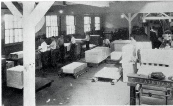
Where much of the unseen work of paper making is carried on. The cutter room, where the rolls of sheets, of all sizes, are run off, cut and packed.
