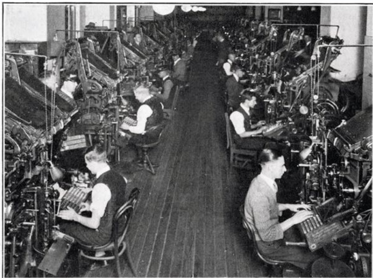
Linotype room, Sydney Morning Herald . A battery of fifty linotypes are included in the Herald equipment.
