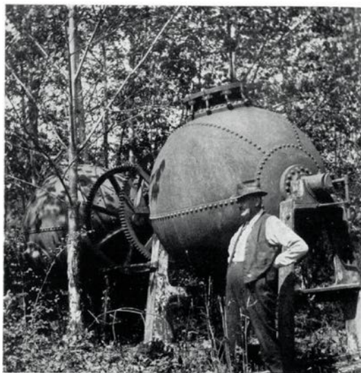
Original revolving digesters of the first paper mill at Alberni, as they look today. Charlie Cox, a resident of Alberni since 1883, is standing by the old machinery.
